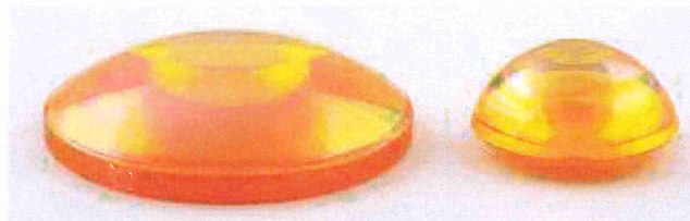
FIGURE 3. Zinc selenide, a commonly used IR optical material, has a large spectral transmission range, but is expensive and not moldable.
