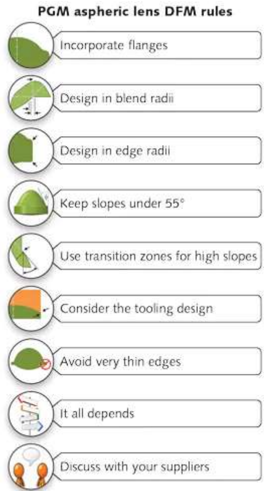
FIGURE 3. Following these PGM design-for-manufacturing (DFM) rules for molding aspheric lenses will help lead to a low-cost, manufacturable design.
